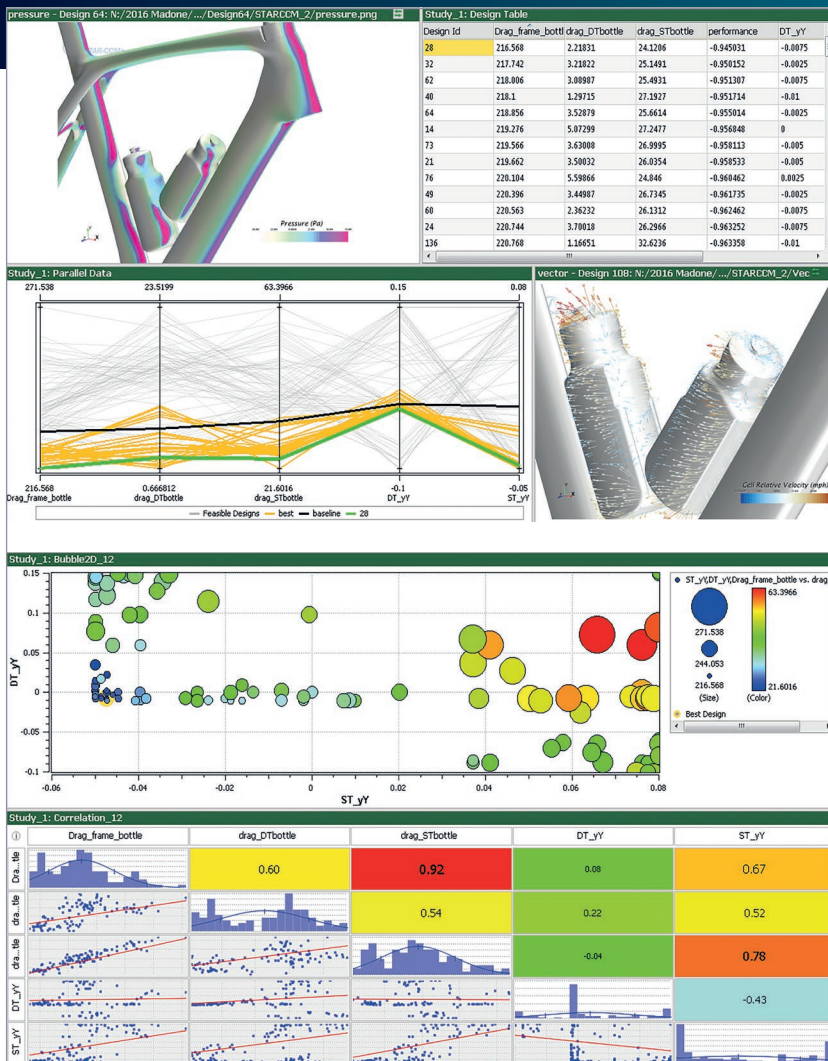
HEEDS output for water bottle placement optimization.
