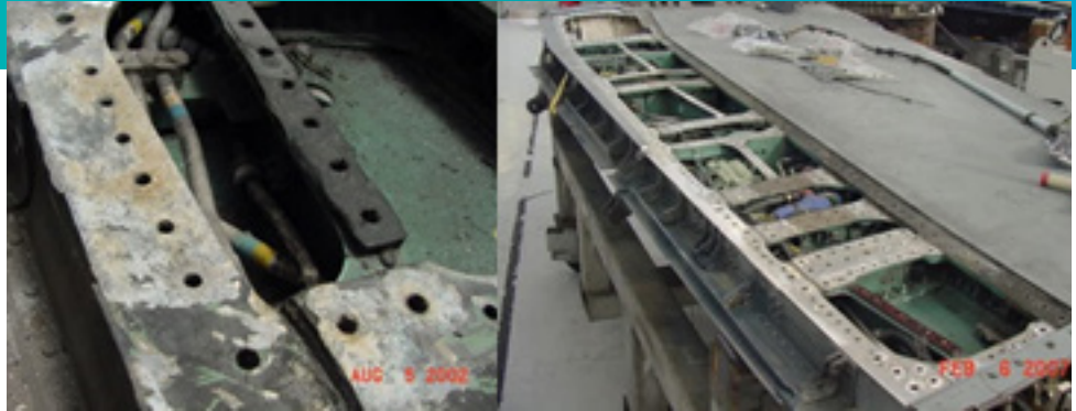
Corrosion on an F-18 wing and airframe.
