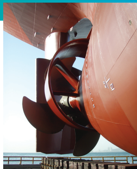
Becker Mewis Duct, "Bow Flora", 37,000 dwt chemical tanker from Odfjell.
