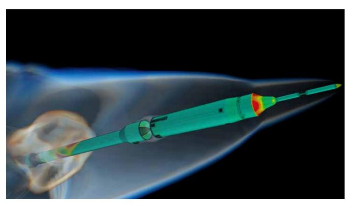
Unsteady simulation of an Ares launch vehicle to understand the aerodynamic characteristics of the stage separation.
