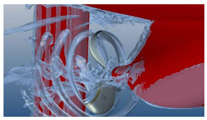
Transient simulation of the self-propulsion of a bulk carrier using the tip modified Kappel Propeller
