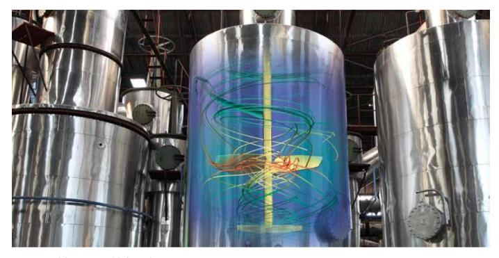
STAR-CCM+ brings automated design exploration and optimization within the grasp of all simulation engineers. Shown here is a mixer design study starting with a baseline (left) and resulting a improved design (right) with a fourfold decrease in power consumption while maintaining blend time. The final prototype is pictured above.
