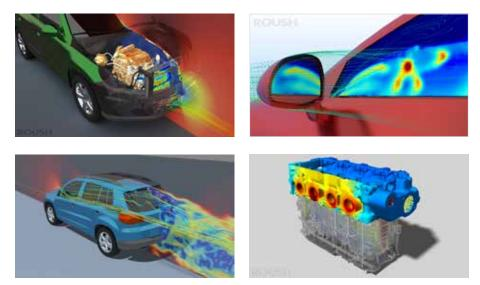
STAR-CCM+ facilitates multiphysics simulations from a single, integrated environment delivering realism in simulation. Shown here is the application of STAR-CCM+ at Roush Industries to tackle multiphysics challenges in automotive product development.
