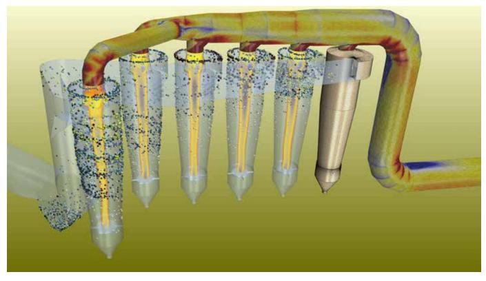
Fluid and particle flow simulation to maximize separation efficiency of a cyclone separator (Image courtesy: Aerotherm).
