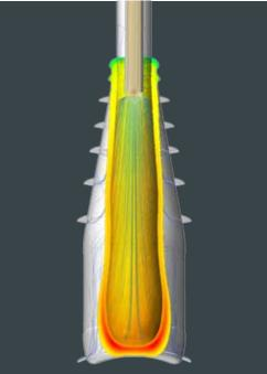
*"We have very complex* physics. The structural and fluid dynamics aspect of the cooling of molten glass cannot be separated because they are very, very, coupled. Understanding the actual temperature of the glass is by far the most important factor in ensuring the strength and quality of the final container. Multiphysics simulation using a tool *like STAR-CCM+ is the* only way that we can achieve that."
