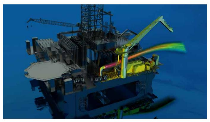
Gas dispersion safety study of an offshore floating platform.
