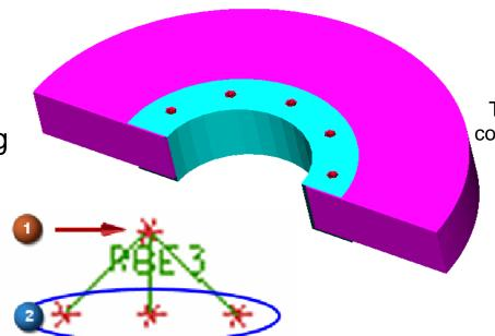
Two constraint elements connected with one rigid bar or beam element
