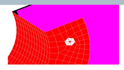
One rigid element connecting all the nodes to one central node
