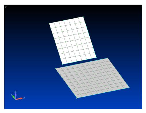
For example, with this model you can see that the two meshed surfaces don't quite meet up, but we can use the Meshing Toolbox to extend one of them and ensure that a final contiguous mesh is created.
