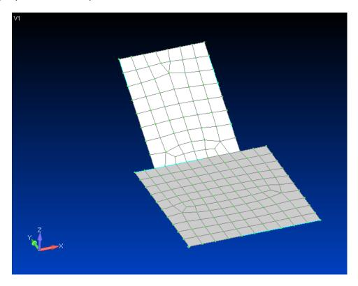
In one action Femap extends the upper surface and the associated mesh and joins the surfaces together to form a continuous mesh across both of them.
