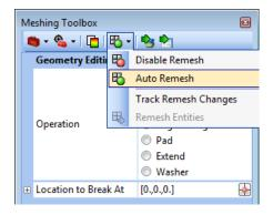
In the Geometry Editing toolbox select **Extend** for *Operation*, and **Solid** for *Extend To*. Then click the **Solid Extend To** icon and select the target solid – the lower of the two plates in this example.
