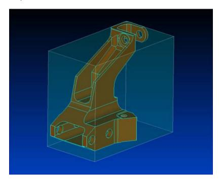
For example, the default tolerance used when merging entities is calculated to be bounding box diagonal divided by by 10,000.
